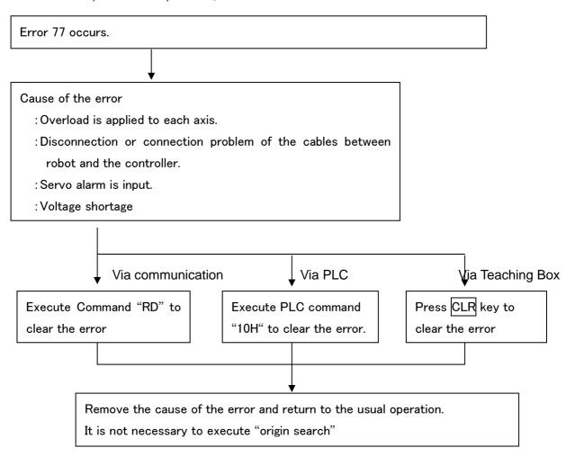
\*Note: Error 77 cannot be cleared depending on the robot specifications. In this case, turn the power OFF and recover.
